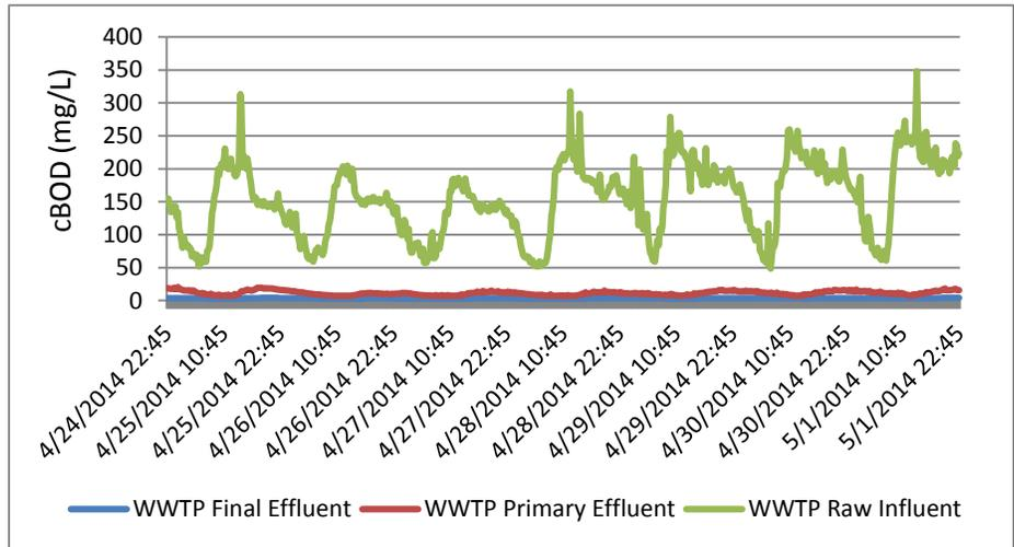
One week of cBOD data from 3 different LiquID HMA Stations positioned throughout a wastewater treatment plant. This graph shows ~4,300 data points per series over a concentration range of 3.1 mg/L in the Final Effluent to 375 mg/L in the Raw Influent.
