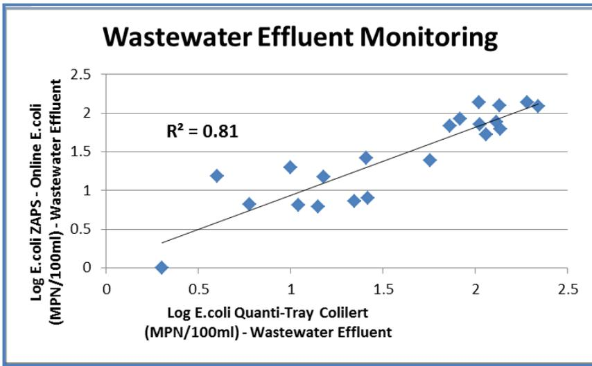
Figure 2B: The same data as in Figure 2A, but plotted as a compilation demonstrating the strong agreement between the ZAPS LiquID output and certified laboratory Quanti-Tray measurements.
