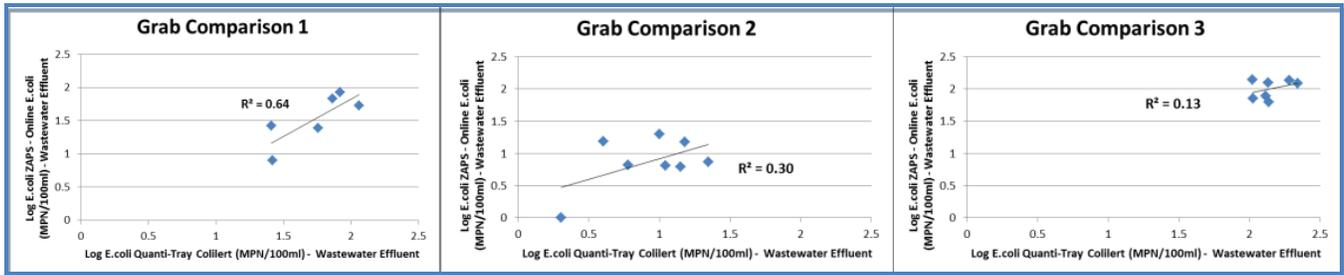
Figure 2A: Data comparing ZAPS LiquID continuous output to certified laboratory Quanti-Tray *E.coli* counts for wastewater effluent samples over limited population abundance. Notice correlations over these limited ranges are equivalent to or better than published duplicate values for the Quanti-Tray method.
