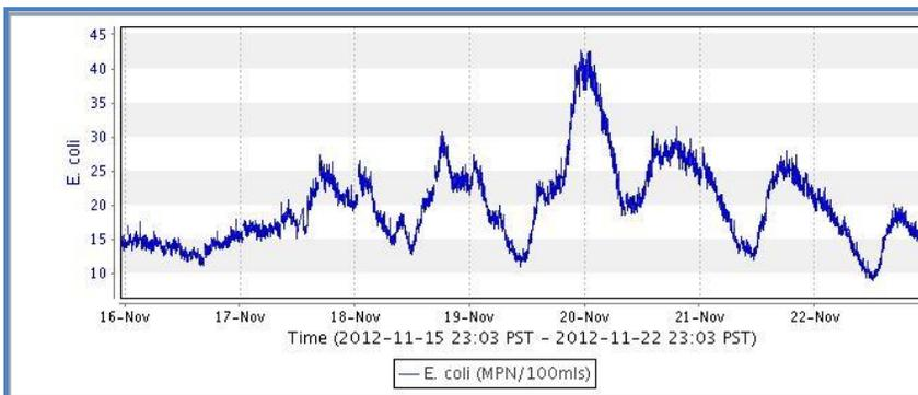
Figure 3: Graphical display of one week of data reported for a signal parameter (*E.coli*) as viewed using the ZAPS Technologies web-user interface (WUI). This one week of data includes 3992 *E.coli* outputs with a geometric mean for the week of 19.1 MPN/100ml.
