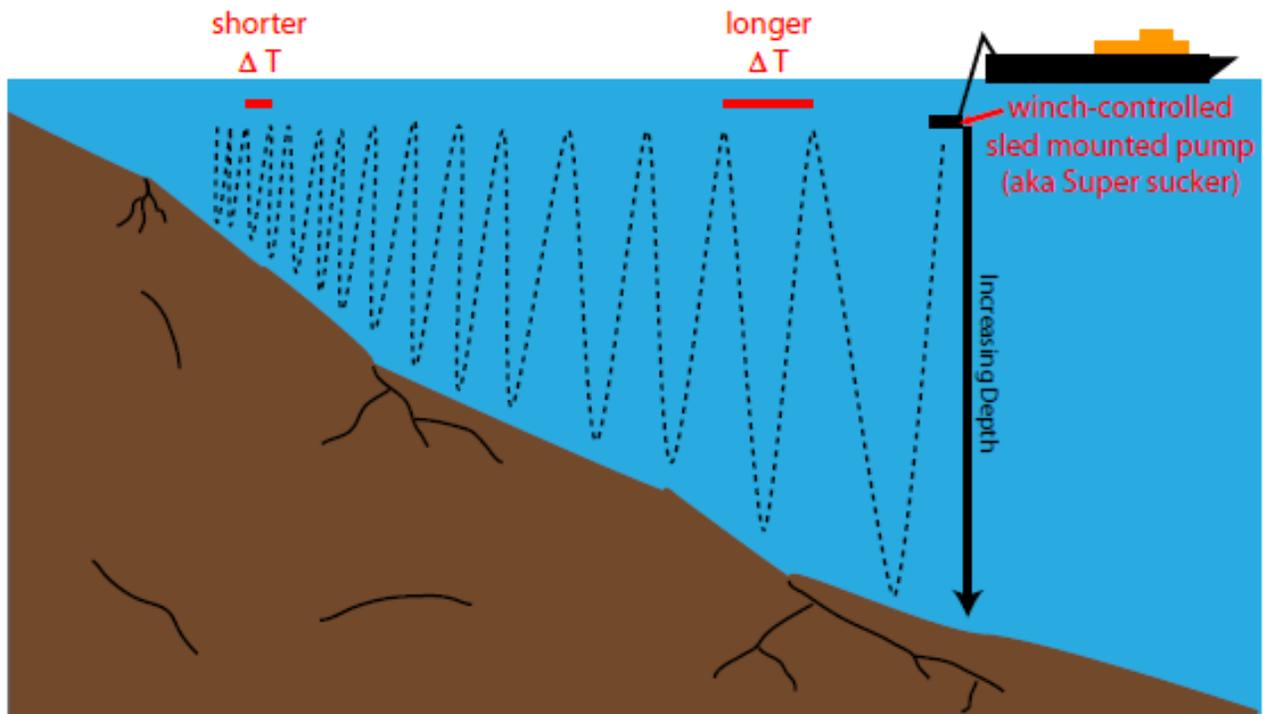
This variation in delta T shows up in the data charts produced by the LiquID station as it analyzes the samples pumped to it from the sled, as shown in the following chart of total organic matter versus time:
