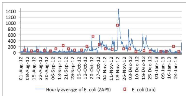
Figure: Comparison of ZAPS LiquID data with conventional lab testing.
