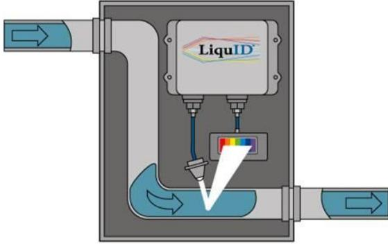
*Above: Stylized view of LiquiD flow-through water monitoring*
