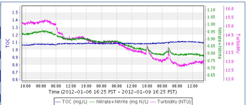
Screen captures of data presented on the LiquidID web user interface. On the left are live, up-to-the-minute readings on the Quick Glance view, while the image above is a 3-day graph using the program’s intuitive graphing feature.
