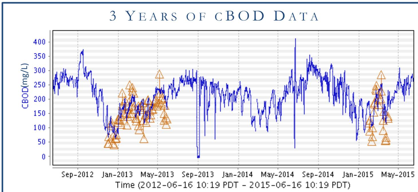
Figure 12: 3 years of cBOD data from a WWTP raw influent location with 8 months of overlaid regulatory data.
