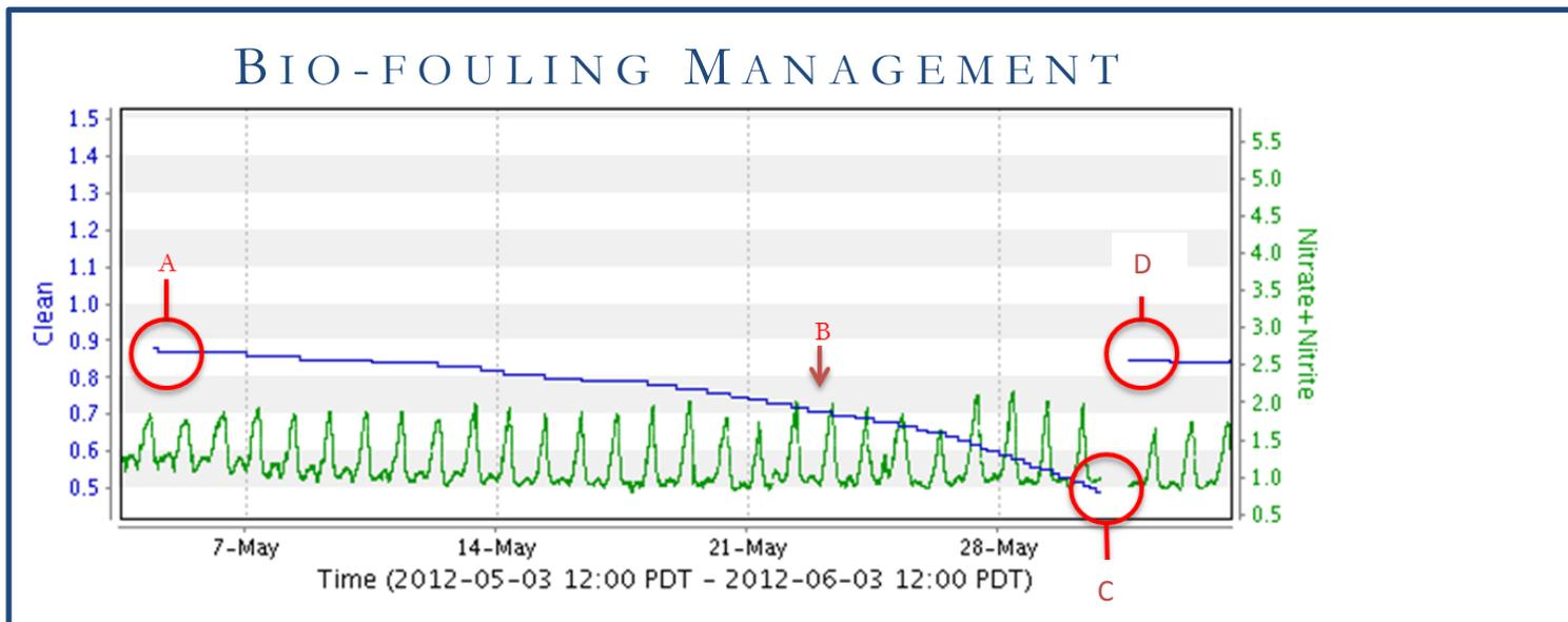
Figure 10: The impact and management of short term degradation (biofouling) management on a LiquiD station.
