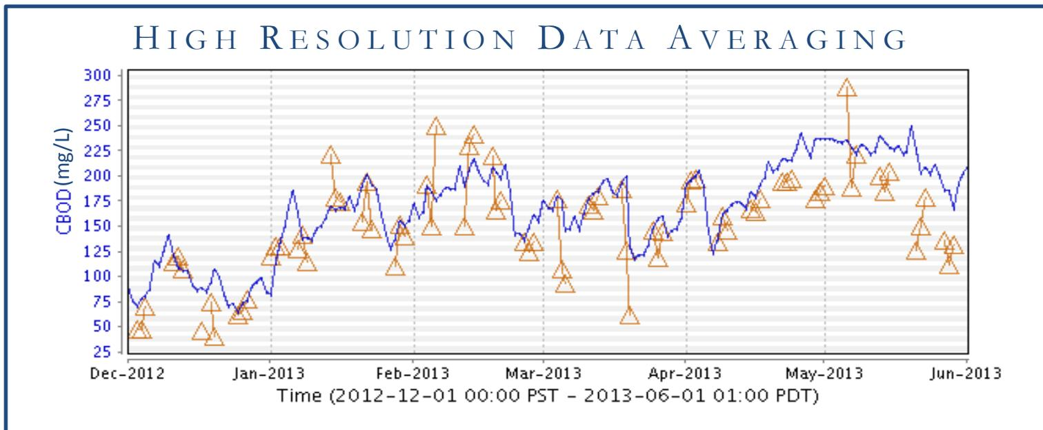
Figure 3: HMA cBOD Daily Average vs Regulatory Composite readings (wastewater influent).
