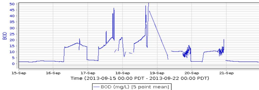
Caption 2: Screenshot from LiquiD. Mid-change. Spikes in BOD show process failure. Sporadic data shows periods when the plant was shut down to address the issue. BOD values during this failure period reached as high as 54.6 mg/L.
