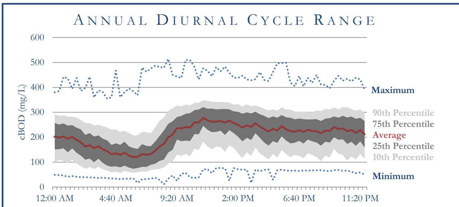
Figure 8: Average cBOD diurnal cycle at a WWTP constructed from one year of real-time HMA data.
