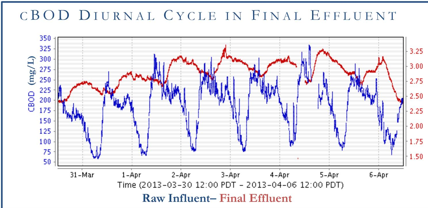
Figure 6: cBOD diurnal cycles over one week compared between Raw Influent and Final Effluent of a WWTP.
