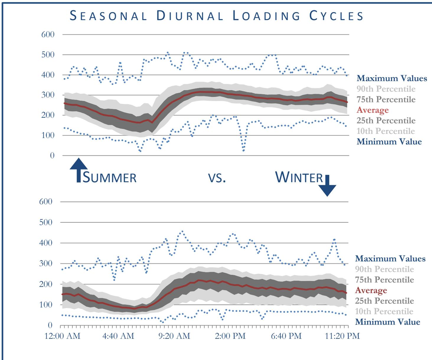
Figure 9: Average cBOD diurnal cycle at a WWTP during summer and winter permit seasons constructed from one year of real-time HMA data.
