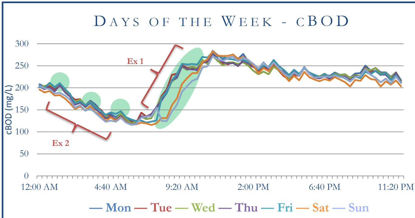
Figure 13: The average cBOD diurnal cycle by the day of the week at a WWTP raw influent location.
