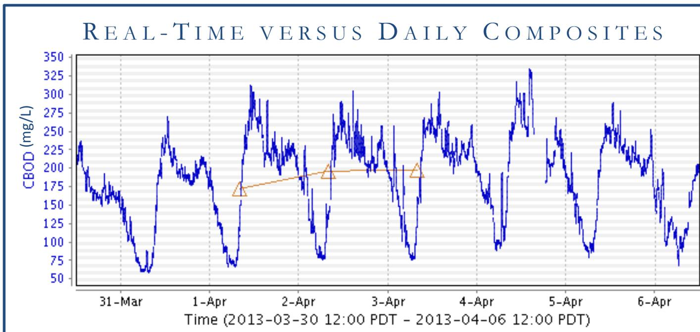
Figure 4: One week of regulatory data (orange) contrasted with one week of real time HMA data (blue).
