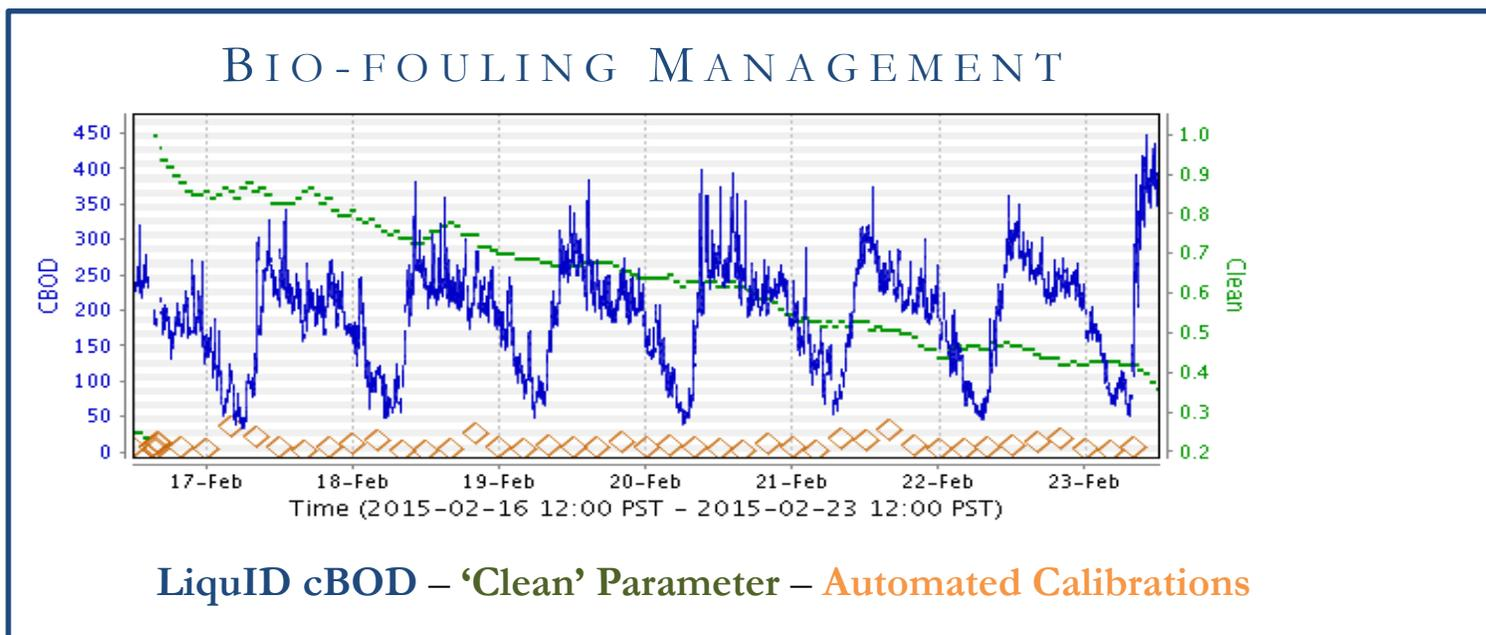
Figure 11: Visualization of the automated calibration and cleaning processes utilized by the LiquID station.
